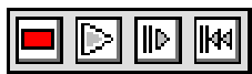
Figure 5. The Control Panel buttons can be used to control the running of the simulation. From left to right, the buttons are "Stop", "Go", "Step", and "Reset". These commands are also available from the Control menu.
